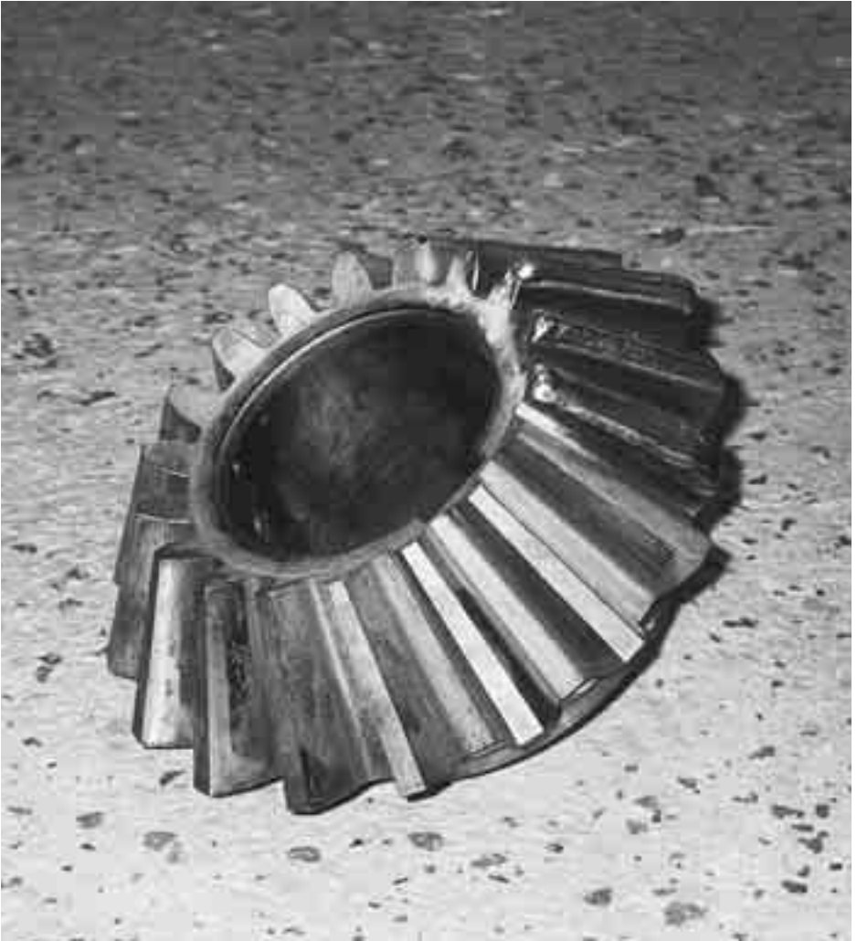
Gear drive. Rebuilding using OK 68.82.
