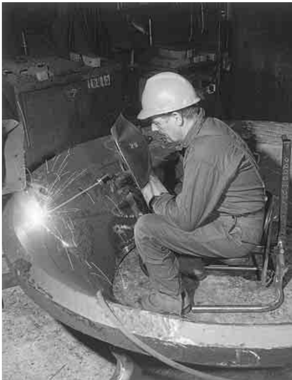
Repairing of 14% Mn steel crusher using OK 86.08.
