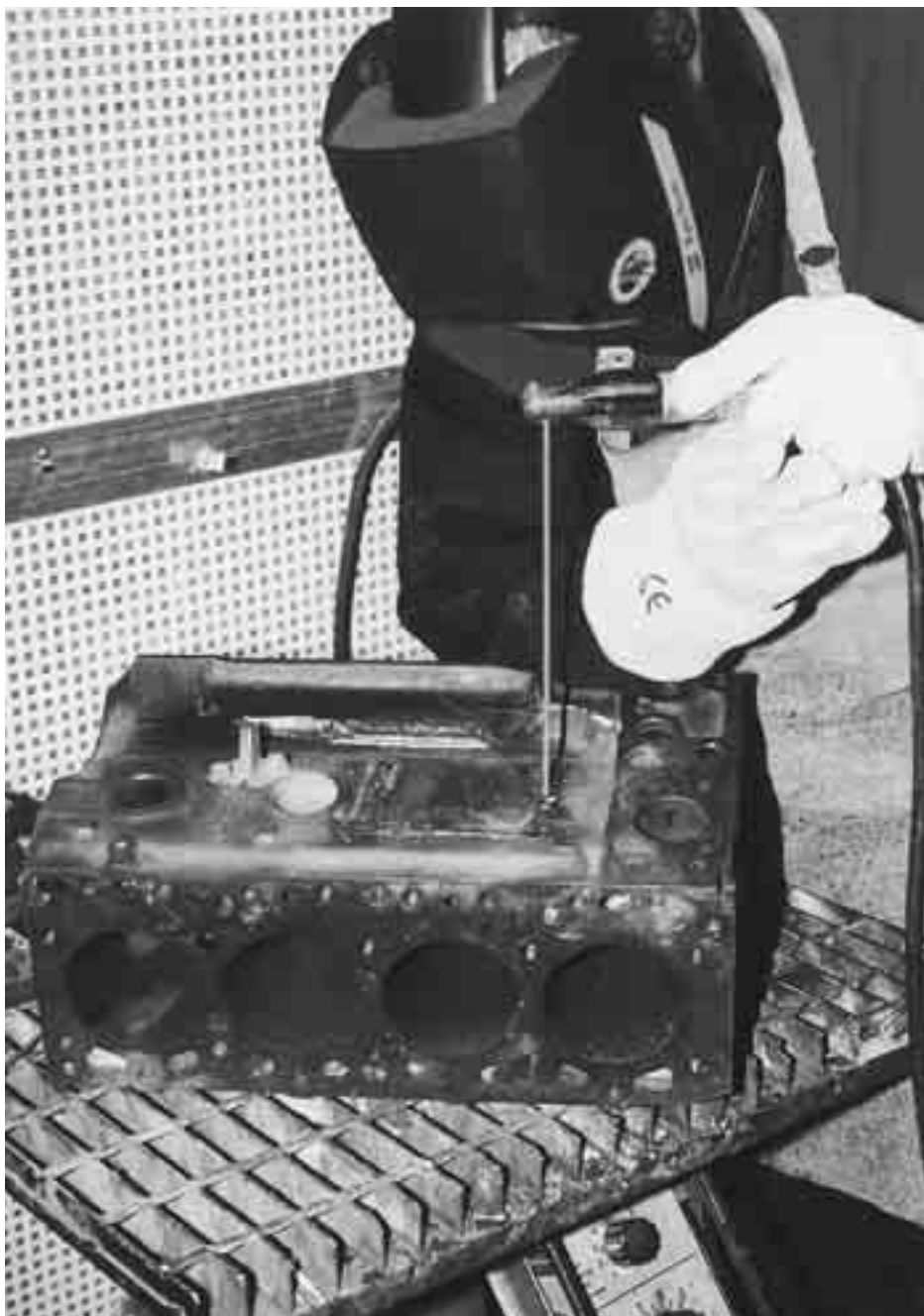
Engine block. Cast iron repair using OK 92.18 and OK 92.60.
