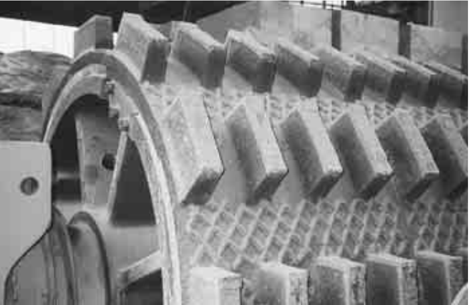
Crusher. Teeth: OK 86.20 buffer layer, OK 84.78 hardsurfacing. Check pattern: OK Tubrodur 14.70.
